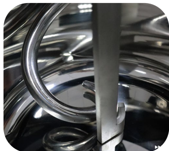
Shaped pasta breaker rod with scraper to collect dough
