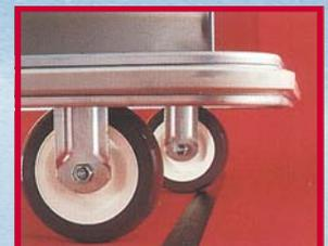
**Wheel-ahead caster configuration.** Makes cabinet easier to move over thresholds and other uneven surfaces, and reduces equipment damage. Heavy-duty polyurethane tread casters resist wear, even on rough surfaces.
