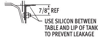
Sectional View Showing Table Connections
