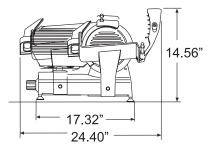
Our slicers have anodized aluminum alloy bodies. The high carbon steel blades are hard chromed, with a hollow ground taper for extended sharpening and blade life. These belt driven machines offer exceptional cutting consistency and durability. The carriage moves smoothly on ball bearings allowing effortless cutting of deli meats and vegetables. Easy to disassemble for quick cleaning. Perfect for low volume operations. Made in Italy.
