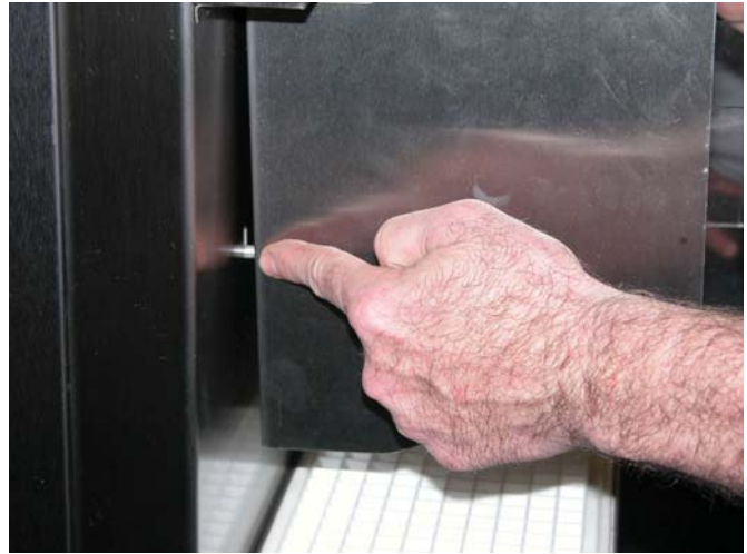
Figure 3-7 Blender Shroud Pin Alignment
