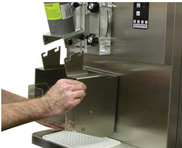
Figure 3-3 Removing Splash Shield Bracket
