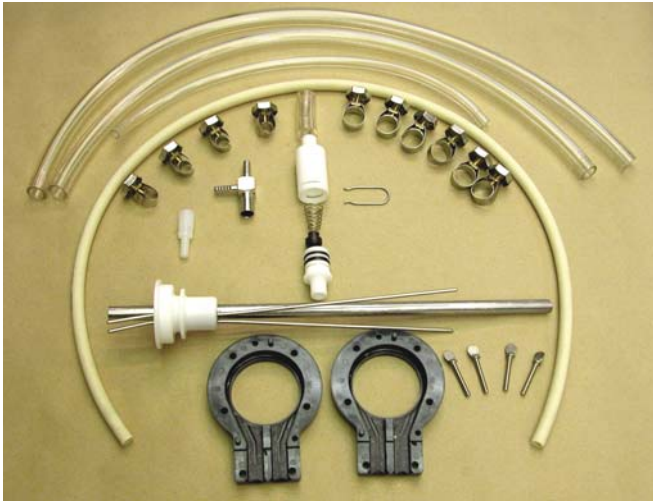
Figure 3-11 Mix Pump Removable Parts
