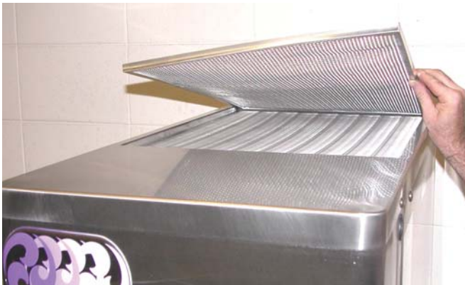
Figure 4-4 Removing Condenser Filter
