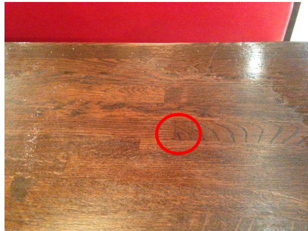
Below: An imported finger jointed end grain with finish failure
