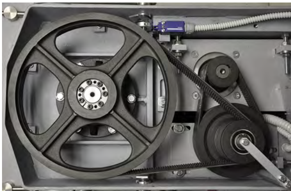
Double reduction agitator belt drive
