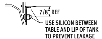
Sectional View Showing Table Connections
