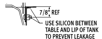
Sectional View Showing Table Connections
