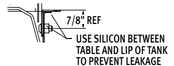
Sectional View Showing Table Connections
