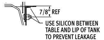
Sectional View Showing Table Connections
