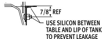
Sectional View Showing Table Connections
