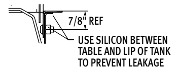
Sectional View Showing Table Connections
