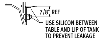
Sectional View Showing Table Connections
