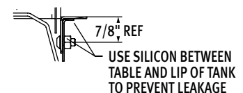
Sectional View Showing Table Connections
