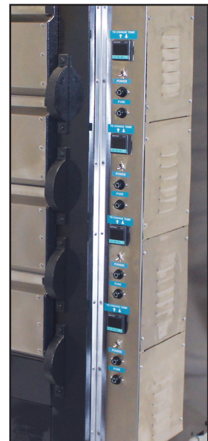
Four control version for better heat control
