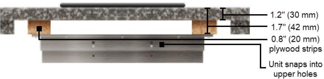
Figure 4-3: Stone Countertop 1.2" (30 mm) with Plywood Strips
