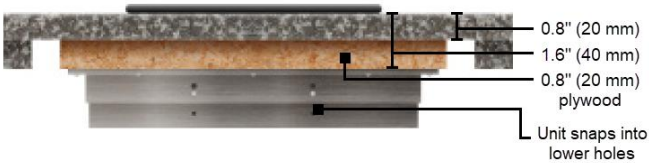
Figure 4-1: Stone Countertop 0.8" (20 mm)
