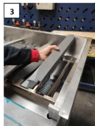
3 TOP CASTINGS ARE REMOVED
