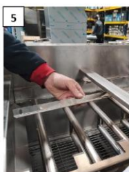
5 BURNER CONNECTION SHEET IS REMOVED
