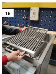
TOP GRILLS INSTALLED
