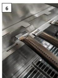
6 BURNER IS REMOVED FROM INSTALLED SHEET
