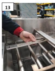
BURNER CONNECTION SHEET IS INSTALLED
