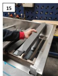
TOP CASTINGS ARE INSTALLED
