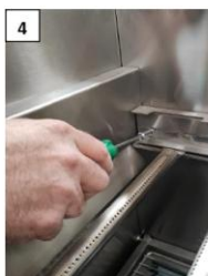
4 BURNER CONNECTION SHEET SCREWS ARE REMOVED
