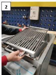
2 TOP GRILLS REMOVED
