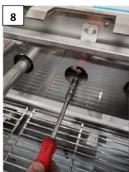
8 INJECTOR IS REMOVED
