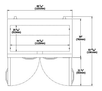
Doors Capacity 13.1 Cu.Ft. Shelves 4 R-290 Refrigerant Temperature -5°F ~ 10°F Range Easy Sliding Condensing Unit Maintenance 9.8 ft long (3m) flexible three Connection wire cord with modeled plug 1/2 HP HP 115V/60Hz Voltage **Amps NEMA Config.** NEMA 5-15
