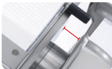
Increased gap between blade and machine body
