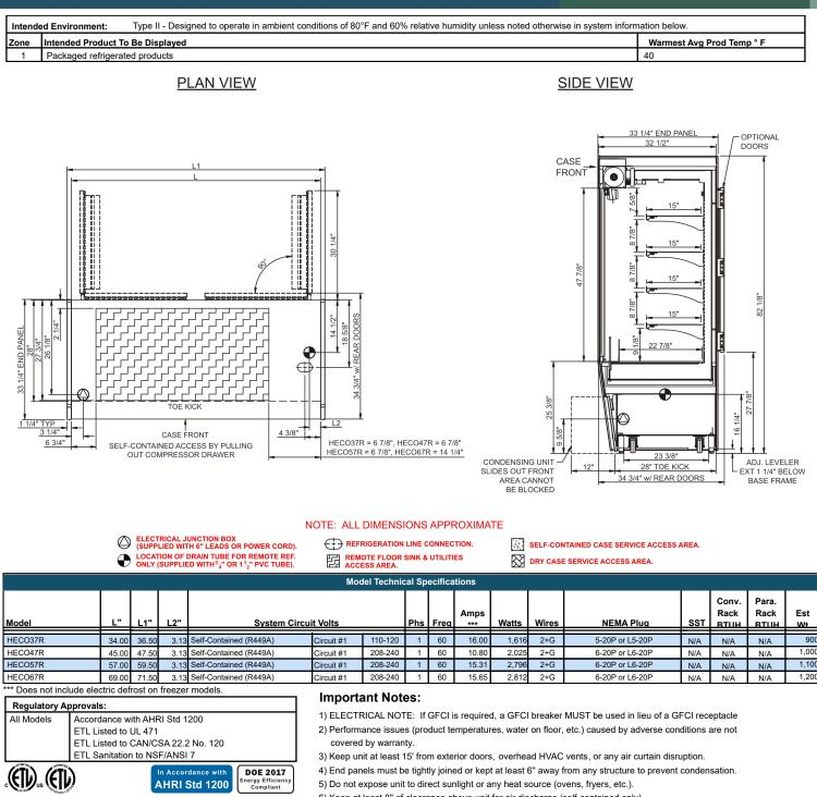
6) Keep at least 8" of clearance above unit for air discharge (self-contained only).
