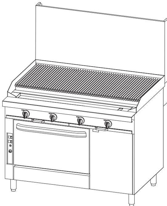
Model P48A-CCCC with optional 24" flue riser
