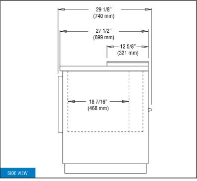
**IMPORTANT NOTE:** Model is completely front breathing and takes in and exhausts air through the front grill. A clearance of 1" on the back and 3" on the sides is recommended.
