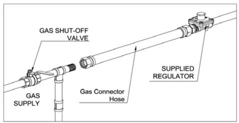
Prior to connecting the regulator, check the incoming line pressure. The regulator can only with stand a maximum pressure of 1/2 PSI (14"WC). If the line pressure is beyond this limit, a step down regulator before the regulator provided will be required.
