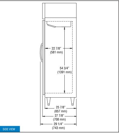
**IMPORTANT NOTE:** If the cabinet is located directly against a wall and/or under a low ceiling, a <u>minimum clearance of 12" is required on top and 3" on sides and rear.</u>
