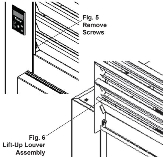
Vacuum or brush any dirt, lint or dust from the finned condenser coil, the compressor and other cooling system parts. If significant dirt is clogging the condenser fins, use compressed air to blow this clear. Care should be taken not to bend any of the condenser fins, as this will reduce performance and compressor life. Lower louver assembly and replace screws to hold it in place.
