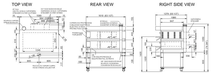
Note: The dimensions indicated in the views are in millimeters. Steamer for Bakery only.
