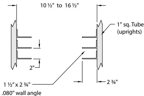
Rack is adjustable on 1" increments.
