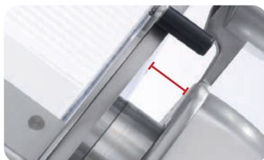
Increased gap between blade and machine body
