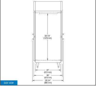
IMPORTANT NOTE: If the cabinet is located under a low ceiling, a minimum clearance of 12" is required on top and 3" on sides.
