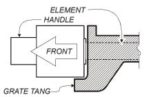
Fig. 5 B-40 GRATE INSTALLATION
