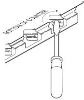
Fig. 3 Set the Wellslloks IMPURIANI: vvater damage caused by failure to set Wellsloks, failure to install gasket, or failure to seal flange to counter is **NOT** covered by warranty.
