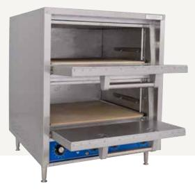
Bakers Pride® P48 series ovens features two independently controlled baking chambers, each with one deck in your choice of Cordierite (7" height) or brick-lined Cordierite (7.5" height). The greater deck height allows you to accommodate taller bake and roast items. The brick-lined model adds a Cordierite ceiling, which offers the benefit of increased temperatures and recovery time. They may be easily installed at the factory or in the field.
